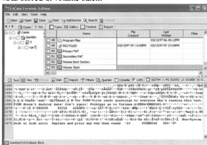
Be aware that a file system may not use an entire partition, leaving space between the end of the volume and the end of the partition, an area called volume slack that can be used to hide data. Figure 8.7 shows remnants of the Form virus stored in volume slack.
